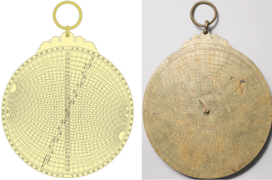
Figures 3a and 3b. The front side of the universal astrolabe. In this drawing, the latitude circles of the Tropics of Cancer and Capricorn are drawn with dotted lines. 34
